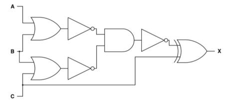
a Redraw the logic circuit using only 4 logic gates. Each logic gate used must have a maximum of two inputs.
